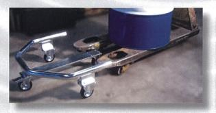
Safe and easy transport of standing drums. The drum can easily be placed or removed from the trolley with a pallet lifter or a truck. The height of the trolley fits an EUR-pallet so the drum can be pulled/pushed to and from the pallet.
