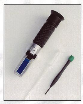
Nimatic Auto Refractometer is securely packed with manual, pipette and screwdriver for calibration.
